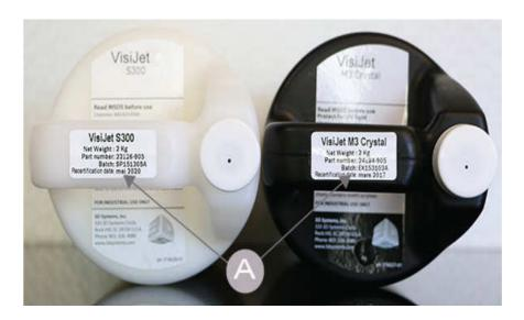
Support (white) material must be loaded in the left side of material drawer. VisiJet part (black) material cartridges must be loaded in the right side of material drawer. Before loading cartridges into printer, inspect the cartridges for signs of damage or leakage. Do not load a damaged or leaking cartridges. Dispose of material cartridge according to local regulations.
