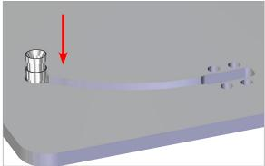
12. Carefully tilt the inner floor at an angle and pull it out of the printer.
