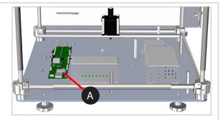
14. Using a 2 mm hex nut driver, loosen and remove the nine (9) 2mm hex head screws securing the Main PCB to the standoffs and remove the Main PCB. Retain the screws for reinstallation.
