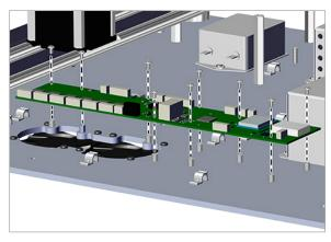
16. Carefully tighten the screws to secure the Main PCB.
