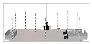
25. Place the heater onto the standoffs and insert the four (4) 2.5 mm hex head screws. Using a 2.5 mm hex head driver, secure the heater to the standoffs.
