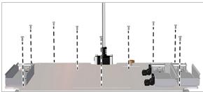
9. Lift the front of the floor plate and carefully disconnect the cables from the cartridge sensors.
