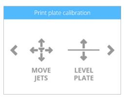
28. Press the up and down arrows for X, Y and Z, and ensure the extruder carriage assembly and the print pad move appropriately.
