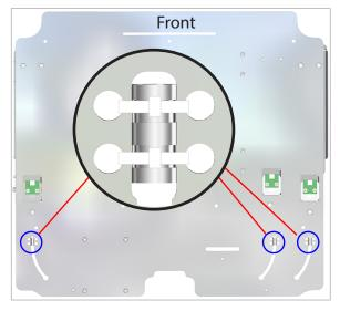
11. Route the delivery tube nuts to the rounded openings in the inner floor and push them through.
