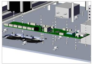
Place the new Main PCB over the standoffs and insert the original screws.
