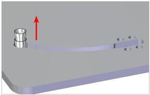
20. Using zip ties, secure the delivery tube nuts to the inner floor. Cut off any excess plastic from the zip ties.
