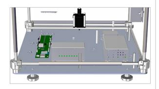
18. While noting the location of the interior heater, carefully place the inner floor back into the printer.
