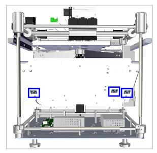
10. Using wire cutters, carefully cut the six (6) zip ties securing the delivery tube nuts to the inner floor.
