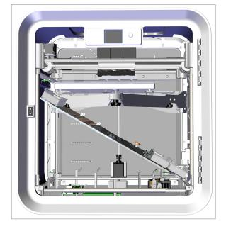
13. Carefully disconnect the wire harnesses from the Main PCB (A).
