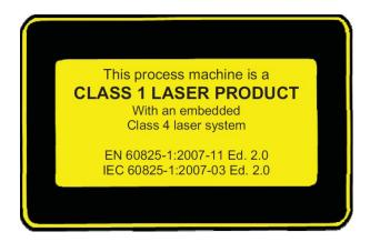
All service to the laser process machine, the embedded laser system and optics requiring interlock override shall only be performed by 3D Systems Corporation service personnel, their authorized agents, or personnel trained by 3D Systems Corporation. The manufacturer's user information for the incorporated laser products are supplied with this process machine.
