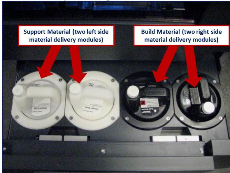
Support (**white**) material must be loaded in the **left** side of material drawer. VisiJet part (**black**) material cartridges must be loaded in the **right** side of material drawer. Before loading cartridges into printer, inspect the cartridges for signs of damage or leakage. Do not load a damaged or leaking cartridges. Dispose of material cartridge according to local regulations.
