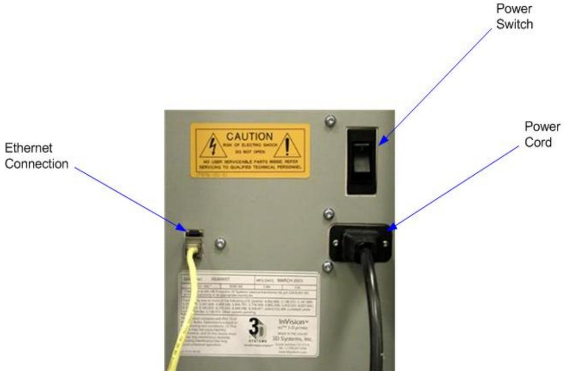
2. When power is restored and stable, switch printer power ON on the rear panel.
