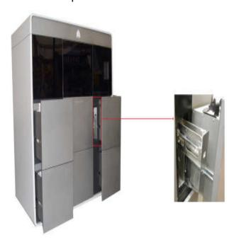
The ProJet® MJP 5600 has two waste drawers, (left and right). The waste drawers are located adjacent to the upper MDMs and can be accessed by opening the MDM. The right waste drawer collects waste from the waste tank and the left waste drawer (not shown), collects waste from the Head Maintenance Station, (HMS).
